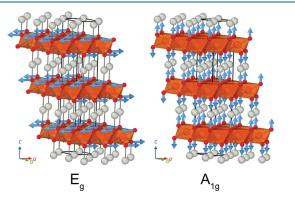
Figure 4. Illustration of displacement vectors describing the two Raman active vibrational modes of  $3R-AgFeO_2$ . Blue arrows represent the displacement vectors of the oxygen atoms for each mode with the  $Fe^{3+}$  and  $Ag^+$  ions remaining at rest. The vector magnitude is arbitrary and scaled only for clarity.
