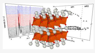
transitions. The high-pressure structure between 6 and 14 GPa is assigned as a monoclinic C2/c structure that is analogous to the high-pressure phase reported for AgGaO<sub>2</sub>. Nuclear resonant forward scattering reveals no change in the spin state or valence state at the Fe<sup>3+</sup> site up to 15.3(5) GPa.
