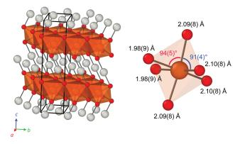
**Figure 5.** Left: crystal structure of the monoclinic C2/c phase solved from high-pressure single-crystal data collected at 6.3(5) GPa. Right: comparison of Fe-O bond lengths and angles in the {FeO<sub>6</sub>} octahedra, clearly showing a distorted local environment compared to the 3R-AgFeO<sub>2</sub> phase. Colors follow the same scheme outlined in Figure 1.
