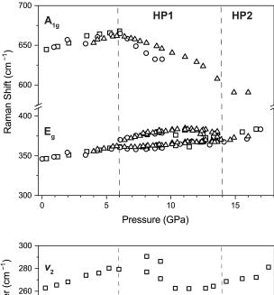
Figure 3. Top: plot of the fitted peak positions in the Raman spectra collected as a function of increasing pressure at 300 K. Different shapes represent data from different crystals. Bottom: plot of the fitted infrared modes selected from the low wavenumber spectra collected at the same pressures as the corresponding Raman spectra above. Dashed lines indicate the pressures at which the total number of resolvable peaks changes, indicating structural phase transitions.
