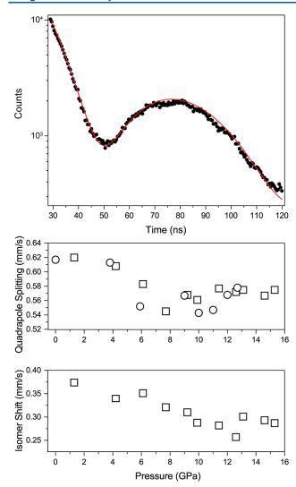
Figure 6. Top: black circles show the NRFS data collected at 0 GPa. The red line shows the fit done by CONUSS that fits the quadrupole splitting as 0.62 mm s $^{-1}$ . Bottom: values of  $\Delta E_{\rm Q}$  and  $\delta$  obtained from fits to the NRFS spectra plotted as a function of pressure. Data from separate experiments are plotted with different shapes.
