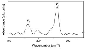
**Figure 2.** Representative Raman (top) and far-infrared (bottom) spectra collected on the same sample of AgFeO<sub>2</sub> at 0.3(5) GPa. Denoted peaks are those whose positions were tracked as a function of pressure. The spectral peak at  $195 \text{ cm}^{-1}$  —which does not move with pressure—is due to diamond birefringence artifacts inherent to the DAC experiments.
