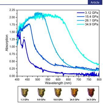
**Figure 7.** Variable pressure UV–vis absorption spectra. These spectra display a feature at approximately 433 nm which grows in intensity and red shifts slightly as pressure increases to 15.4 GPa (top). Above approximately 19 GPa, the features widens to give one large, flat feature in the UV and visible regions. The starred feature is assigned as the  ${}^{6}A_{1g}$  to  ${}^{4}E_{g}{}^{4}A_{1g}$  transitions. The single crystal of jarosite exhibits piezochromism (bottom).
